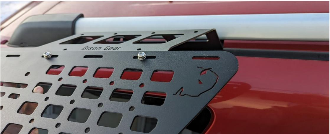
5. Align the T-Bolts with the holes in the panel bracket
