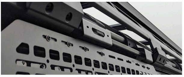
Attach the panel to the car. On top use 6 M6 bolts (two per bracket).
