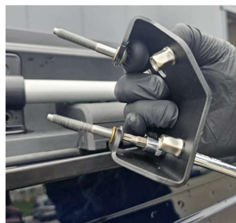
3. Screw **the wind deflectors** to the panel using **M5x12 flange bolts**.
