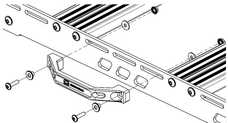
Use 2 **M6x25 Flange bolts** included in the set, add the adapters to make the holes in the Grab Handle smaller, on the other side **remember to add the washers** before screwing the nut.
