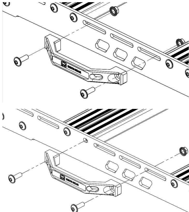
You can attach the handle anywhere along the railing using 2 **M8x25 Flange bolts** included in the package or you can fix one side of the handle using a bolt that mounts the profile to the railing.
