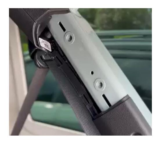
2. Mount  ${\bf right}$  and  ${\bf left}$  bracket using  ${\bf M8x25}$  bolts in factory covers place.
