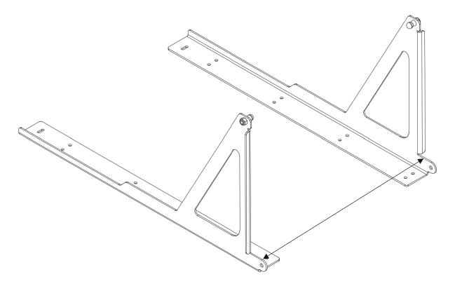
Next, put the slider between holders. Space between the holders and slider fill using M8 plastic washer (should be 1-4 plastic washer). Screw the bolts and tighten them till the slide can smoothly rotate.
