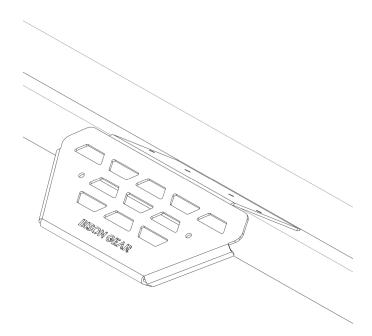
3. Pre-screw **all brackets** according to the diagram, using **M6x16 bolts** and **M6 nylon flange nuts**.
