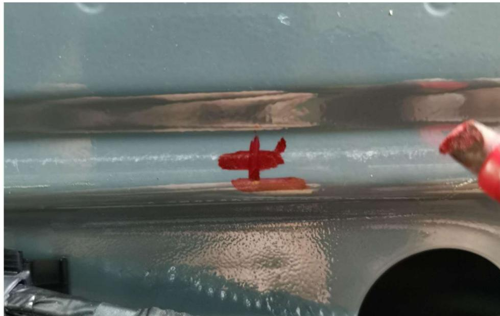
4. Drill the holes in the marked spots first with a small diameter drill bit (ex. 2 or 3 mm) then with a 9 mm drill bit.
