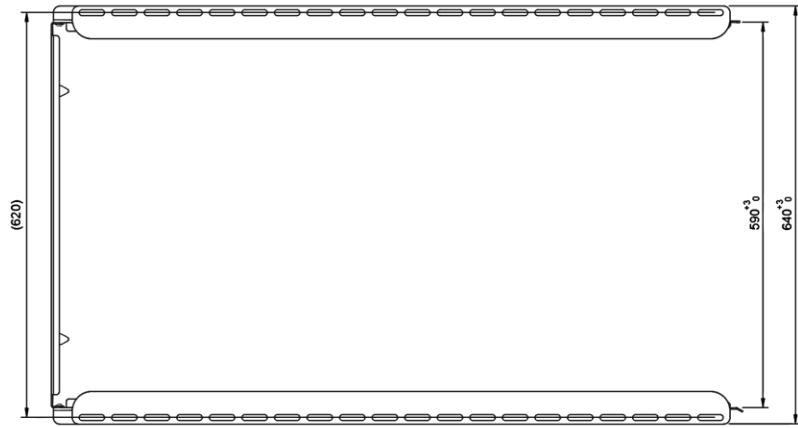
E. Slide the table into the previously assembled guides and close using table closing part (regulate the latch – if it necessary ).
