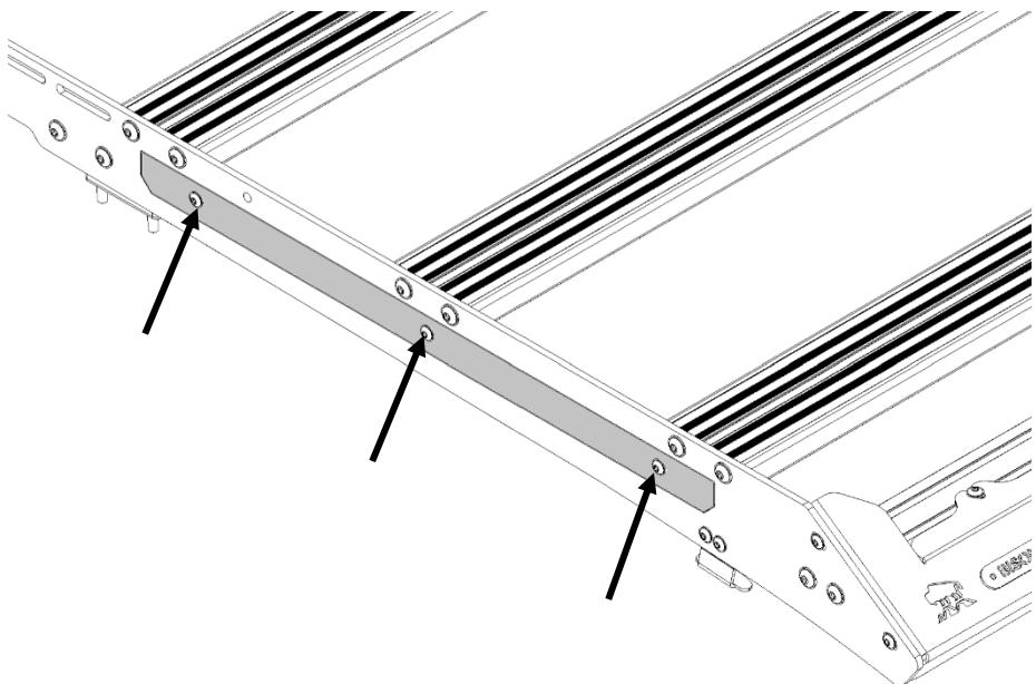
B. Remove the support bracket (unscrew the three M8 flange nuts).
