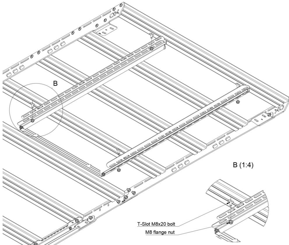
II. Check the dimension with the following drawing. Regulate if it necessary and tighten the nuts.
