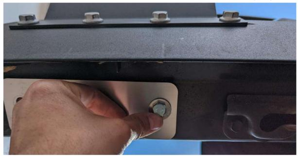
Place the bolt from the bottom of the doors through door skin and inner support. From the inside of the doors place washer and nut. Align support plate. Tighten both bolts.
