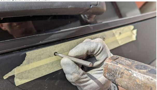
5. Drill holes, start from a small drill bit (~3 mm) or use a step drill. Use an 11 mm drill for the final hole.
