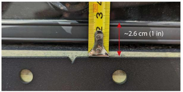
Distance from the top edge of the rubber seal should be around 2.6 cm (1 inch).
