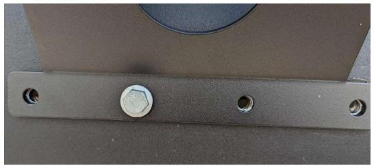
17. Tighten all bolts on top and then on the bottom of the wheel carrier. **Torque to 65 Nm.**
