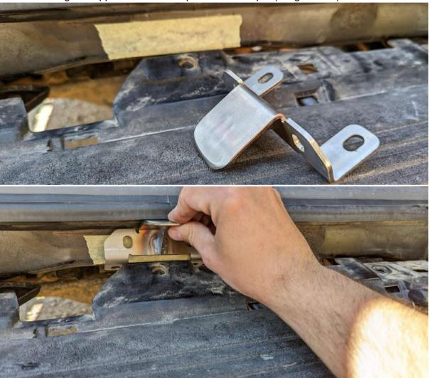
26. Mark hole position. Drill in the bottom part of the slot.
