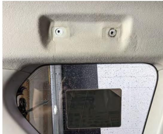
2. Remove **plastic cover** under the trunk window.
