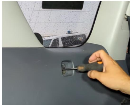
4. Use a **long bolt** and **spacer** to attach a lower bracket to the car.
