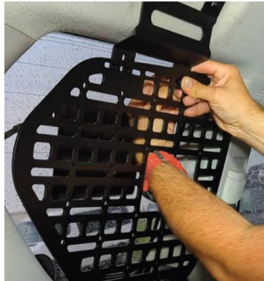
7. Use two **M6x16 bolts** to attach the panel to the bottom bracket.
