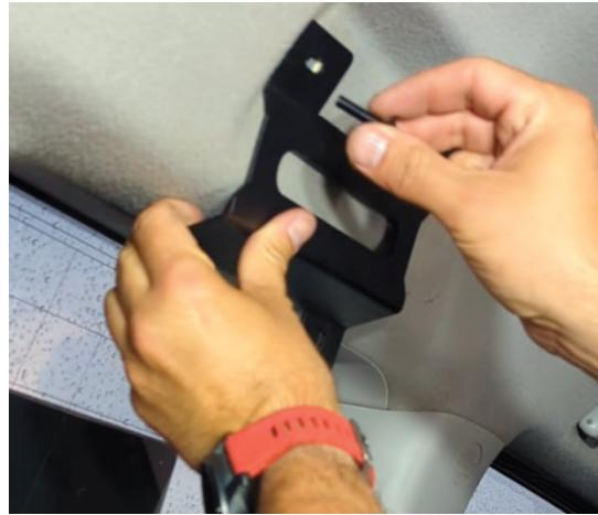
6. Use two **M6x12 bolts** and the **nuts** to attach the panel to the top bracket.
