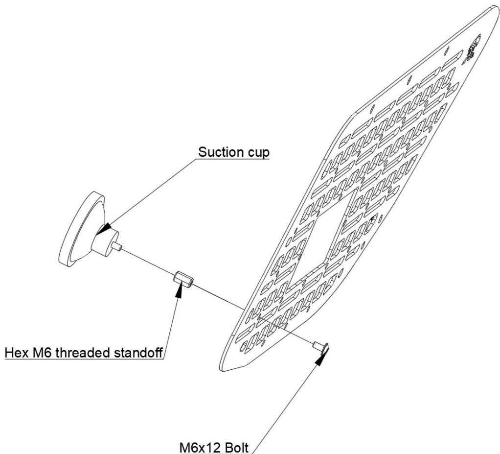
5. Attach the suction cup to the Panel using hex M6 threaded standoff and one M6x12 bolt
