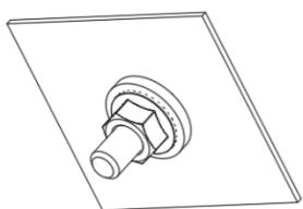
After clearing the way for the assembly process start with attaching the T-bolt to your car's chassis as shown on the diagram above:
