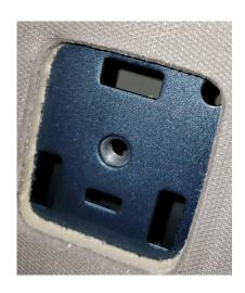
2. Drill a **22-millimeter hole** in each cover as shown below (the hole must be in line with the threaded hole under the plastic). Use a **step drill** or **two drills**, first a small one (**3-5 mm**) for the pilot hole and secondly, a **22 mm** or %" drill for the final hole. It's possible to install the panel without the covers; in that case, drilling is not required. Mark the position of the upper bracket's oblong holes on the car body. Make sure that the marked position is correct.
