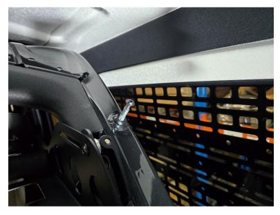
The direction of the sleeve is very important. It should be inserted so that the metric thread is on top. The sleeve should also be inserted approximately 10 mm under the top of the hole (photo below).
