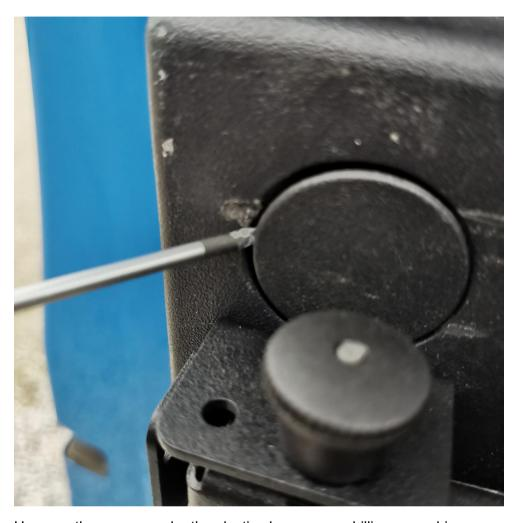
Unscrew the screws under the plastic plugs, use a phillips screwdriver.
