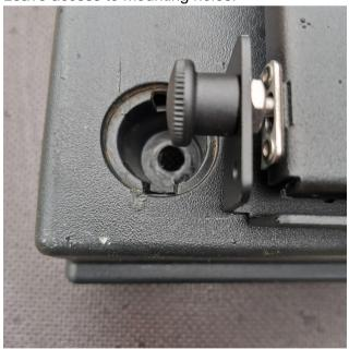
Using holes in the front panel mark holes using small drill bit or sharp pick.
