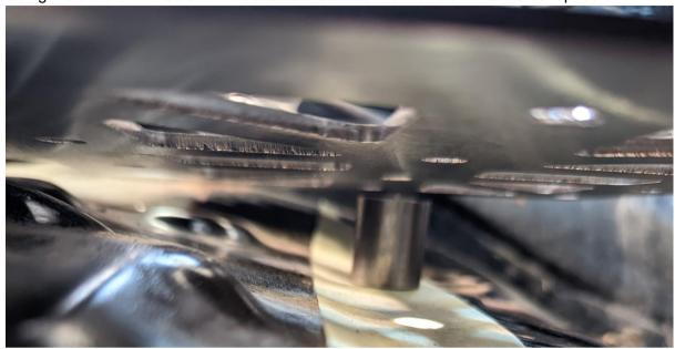
6. Mark center of the slot on the fender "C"
