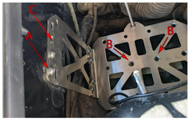
2. Test fit battery bracket. Screw in M6 bolt in place marked by "A"
