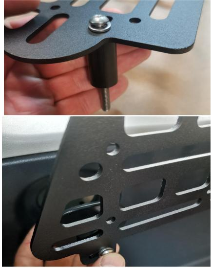
6. Tighten all bolts after aligning the panel properly.
