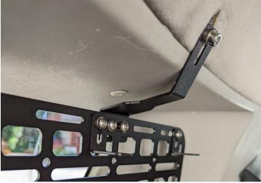
5. Using factory hooks, large plastic spacers, M6x60 bolts and washers attach panel in the bottom.
