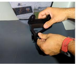
5. Use M6x20 bolts to attach the upper bracket.
