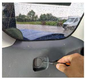
3. Unscrew bolt, using 10 mm socket or philips screwdriver.
