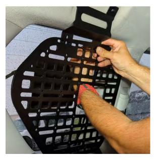
7. Use two M6x12 bolts to attach the panel to the bottom bracket.
