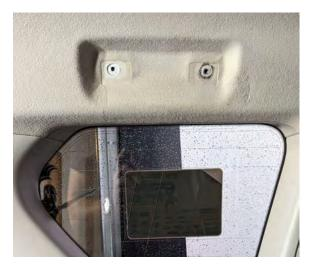
2. Remove plastic cover under the trunk window.
