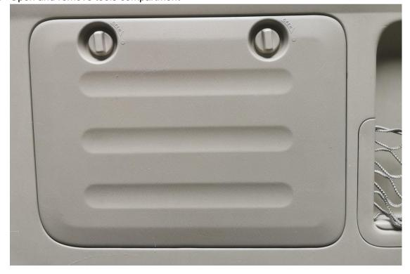
7. Gently pry the trim on right bottom corner, using flat screwdriver or trim removal tool
