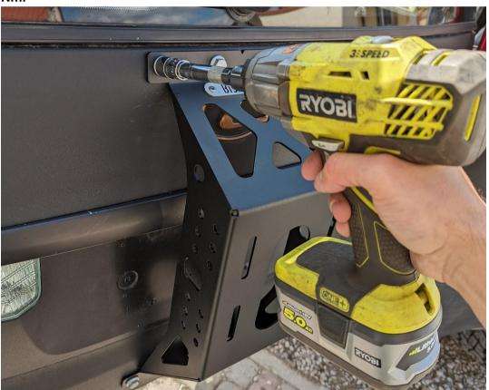
18. Drill 8 mm holes in the back skin of the doors. Hole placement is on edge of the bracket that keeps the door handle. It should go through the door and the bracket
