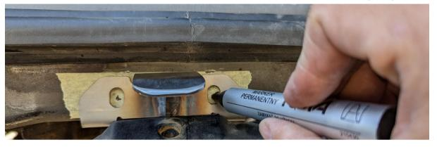
27. In marked spots drill holes with step drill or using small drill bit got to the final 11 mm bit.
