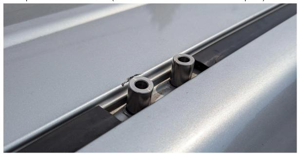
3. Bolt on all brackets. Use a long M8 x 55 mm bolt, M8 spring washer, M8 flat washer (the bolt head might be different than in the attached photo). Leve bolts loose for further adjustment.
