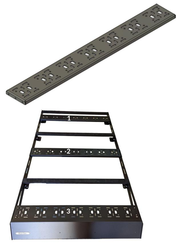
3. Using M6 x 20 mm bolts, spring and flat washers, attach bars in preferred positions.
