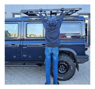
12. Attach the Roof Rack to the small brackets previously installed on the car using M6x16 bolts. It is important to note that power tools should not be used, and the bolts should not be tightened until all 24 bolts are manually screwed in.
