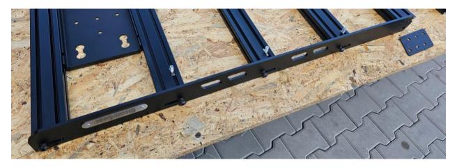
4. Fit the connecting plate, ensuring alignment with the side bar.
