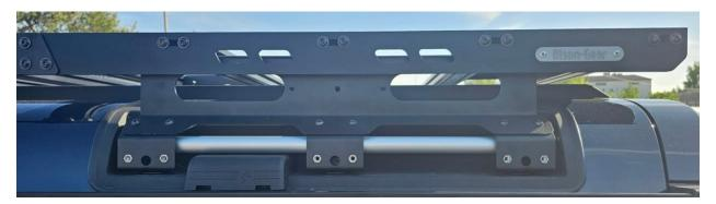
13. Ensure the Roof Rack is properly aligned, then proceed to tighten all bolts.
